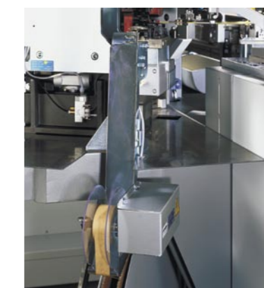
Terminal feed with carrier strip take-up unit
