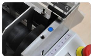
The machine can not be started when the protective cover or cover of the spout is open. A corresponding error message is displayed on the display, which must be cleared with the STOP key.
