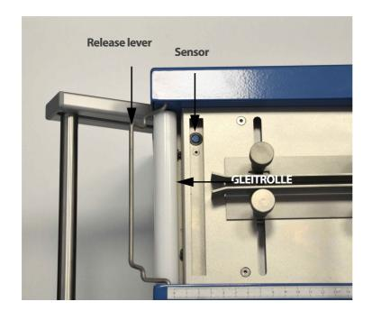
The material to be cut must be fed over the guide roller.
